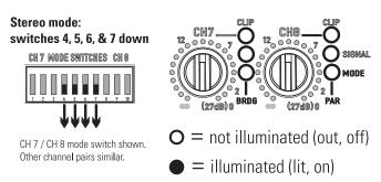
Mode switch settings and LED indication for stereo mode operation. BRDG and PAR indicators should not be illuminated when in stereo mode.
